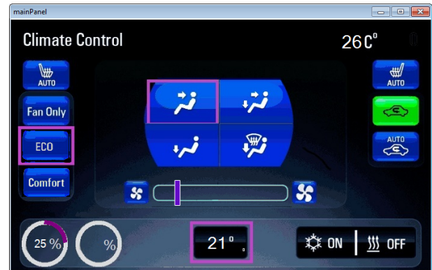
Figure 7: A screen-shot of the GUI with advice from CARE. Note that the advice is shown in purple. The left purple circle represents the expected energy consumption from following the advice. The right circle represents the current energy consumption is empty, since the driver did not yet turn on the climate control system.
