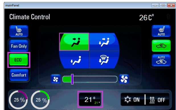
Figure 8: A screen-shot of the GUI when the driver set the climate control system to match CARE's advice. The right green circle represents the current user energy consumption and the left purple circle represents the advice's expected energy consumption.
