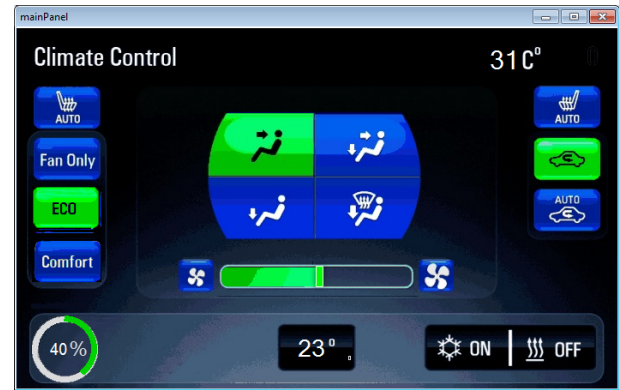
Figure 5: A screen-shot of the GUI with additional energy consumption information provided by CAREless (the circle in the bottom left corner).
